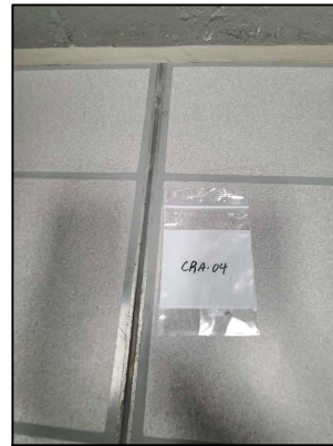
6. View of non-ACM containing flooring seam caulk sample CRA-04 located in the men's side maintenance room; brochure room.
